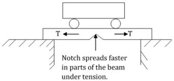
The beam breaks easily when the car crosses the bridge because the notch is in the region of tension and therefore it weakens the beam.
